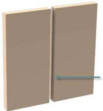
*Important tip*: In construction projects - be it new construction, major renovation or retrofits - installers may encounter wall conditions that are less than true. Specifying solid surface panels with an s-curve "wavy" edge allows panels to fit together with a flat, flush seam where the wall may fluctuate.
